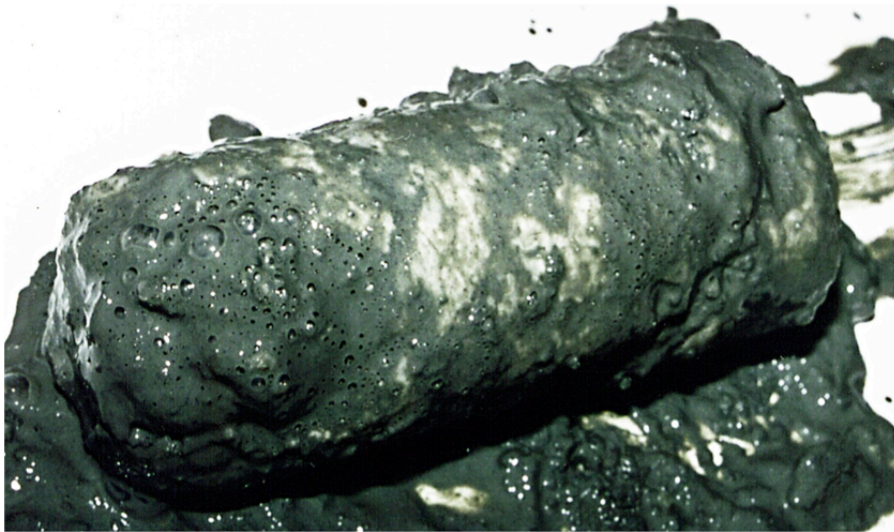
Figure 3. Photograph of a nearly pure piece of gas hydrate (Section 164-997A-42X-3; 331 mbsf) that is ~5 cm × 14 cm in size, white colored, and coated by greenish gray drilling slurry. Note the bubbles within the slurry.
