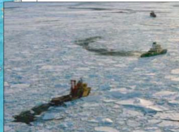
< An example of an MSP operation (Expedition 302) in the Arctic. The first Arctic coring expedition (ACEX) was conducted from August to September 2004, at the crest of the Lomonosov Ridge in the central Arctic Ocean (left). The Vidar Viking drill-ship (right) was protected by two icebreakers Oden and Sovetskiy Soyuz . Vidar Viking drilled five boreholes at four sites, and a 339-m [892-ft] long sedimentary sequence was recovered in the cores. (Photograph courtesy of M. Jakobsson, IODP)
